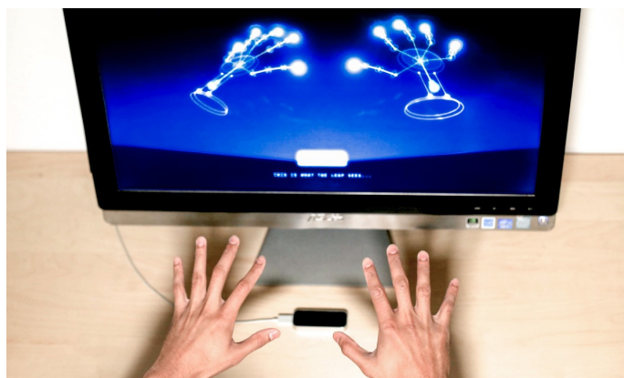
Figure 1: The Leap Motion in use, with onscreen graphic representation of data generated
