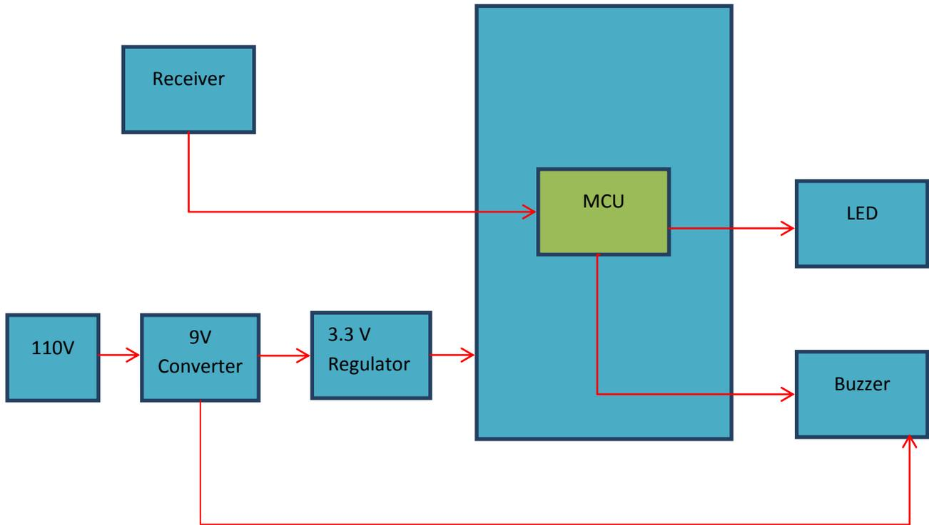
**Figure 9: Receiver Hardware Diagram at Level 0**
