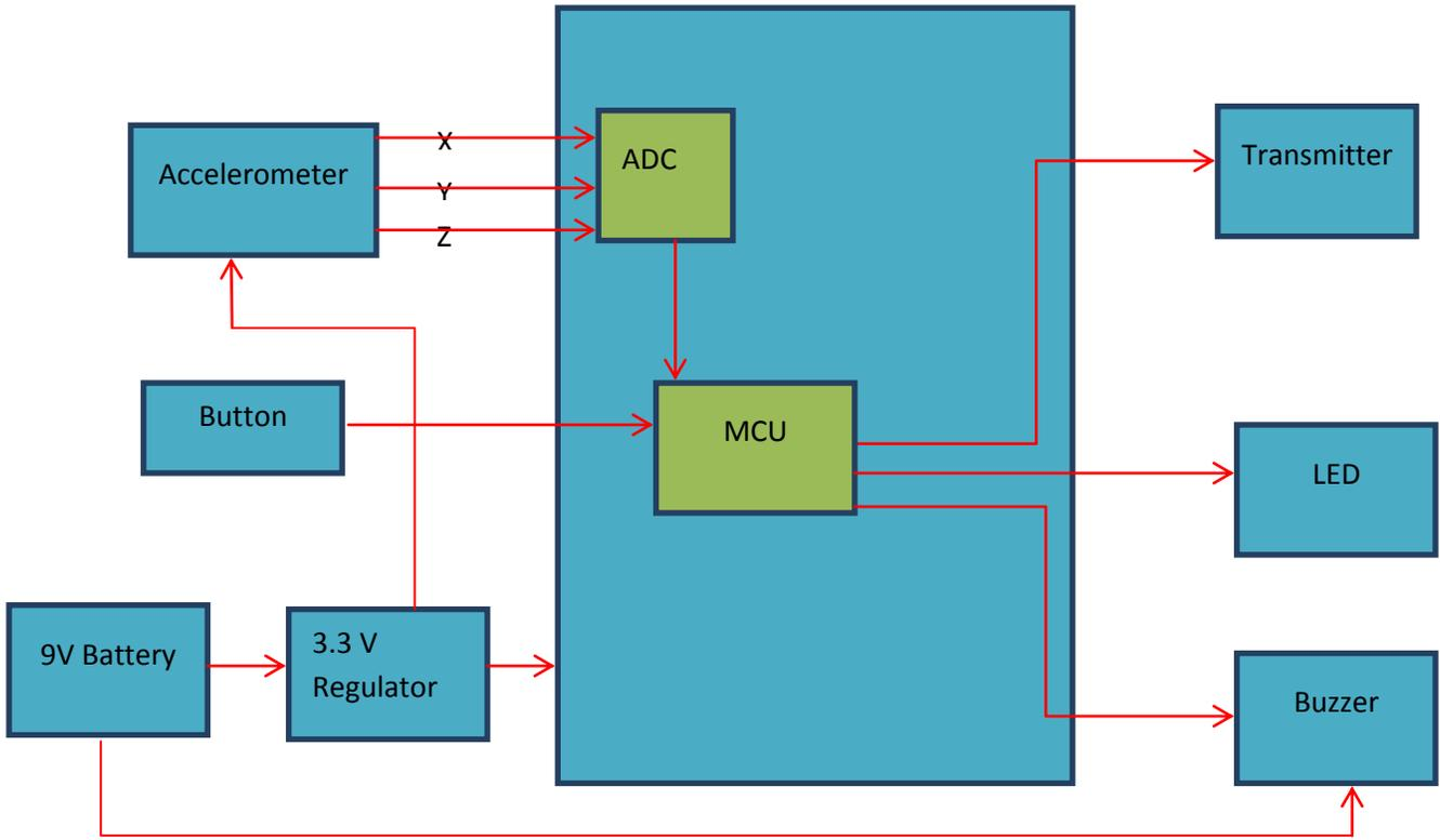
**Figure 8: Transmitter Hardware Diagram at Level 0**
