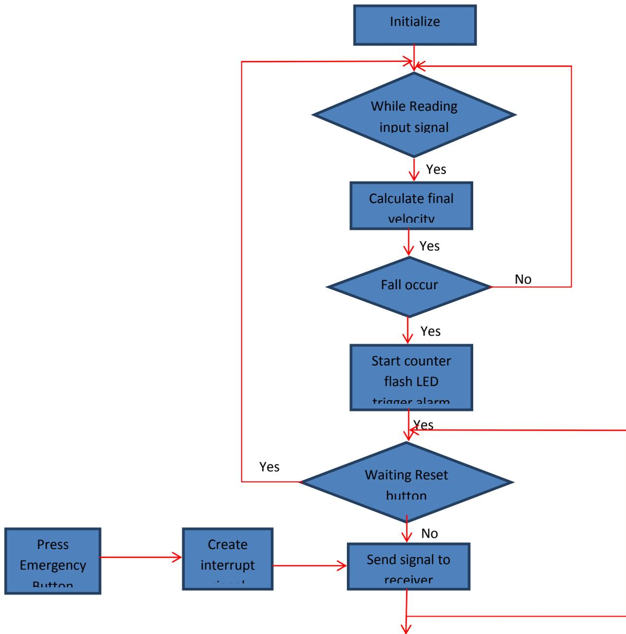
Figure 12: Transmitter Software Diagram
