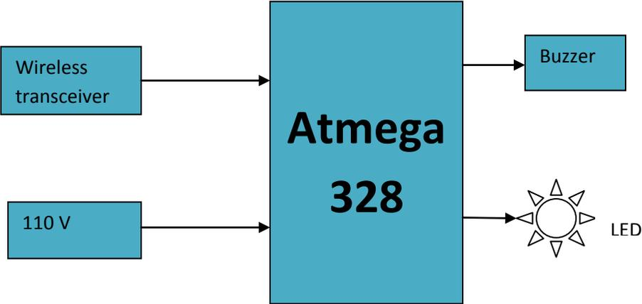
**Figure 7: Receiver Hardware Diagram**
