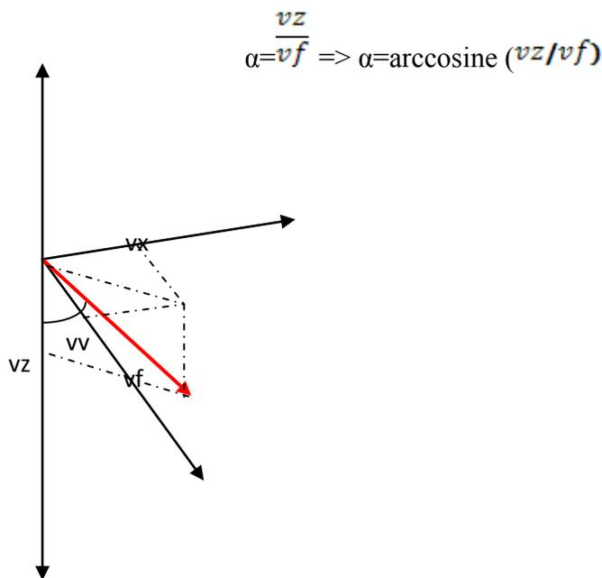
Figure 1: Accelerometer vector
