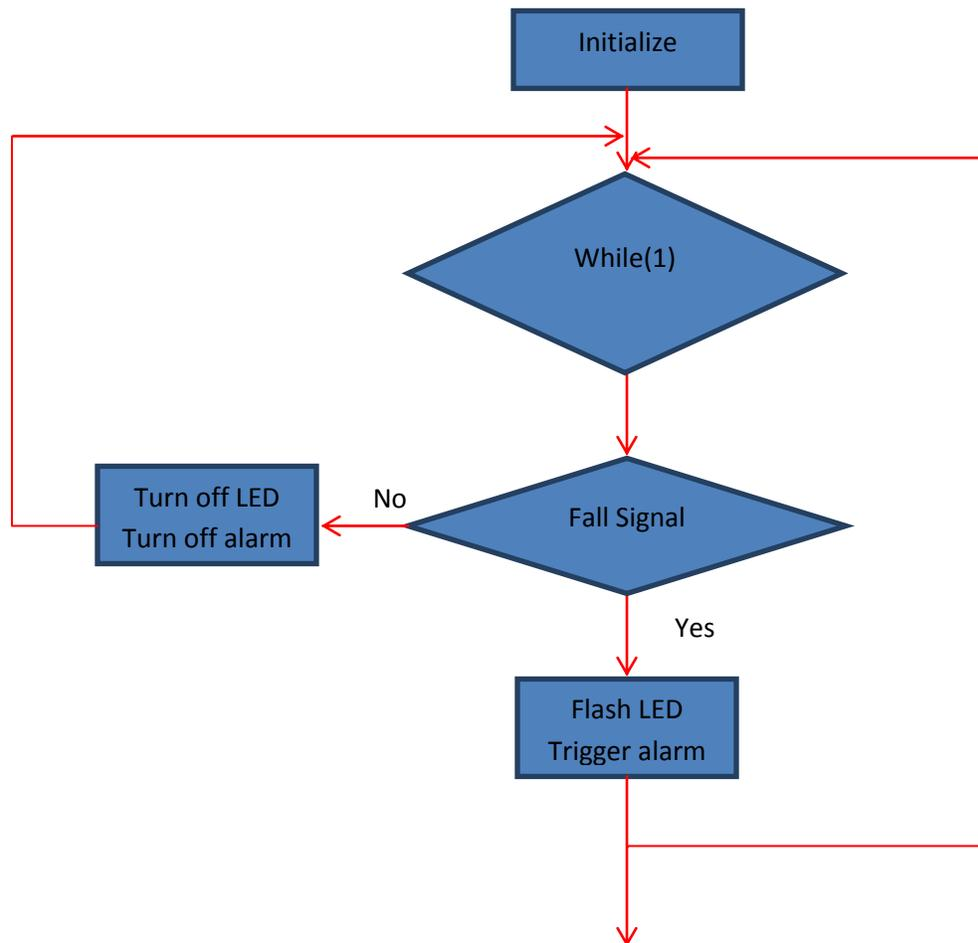
**Figure 13: Receiver Software Diagram**
