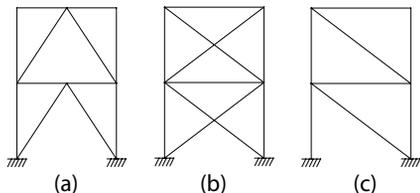
*Figure 2: Examples of concentrically braced frames.*
