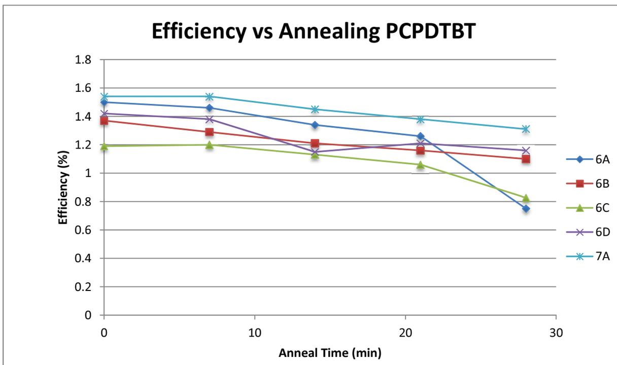
Figure 3b - Efficiency testing for PCPDTBT devices at 140 °C for 7 minute intervals. Devices all seem to drop from annealing, these results were not reproducible in the second PCPDTBT run but this may have been caused from an overly dissolved polymer layer or the higher temperature anneal.
