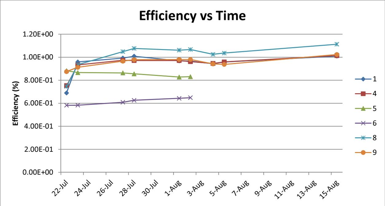
Figure 5a – Shows the efficiency of PCPDTBT and P3HT:PCPDTBT devices from the second run through time. Devices 5 and 6 were removed from the graph early because they were annealed. The rest of the devices can be found in Table 6.
