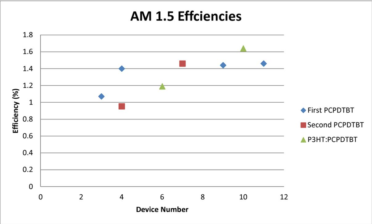
Figure 8 – Different devices from the first and second runs. Devices efficiencies were averaged over device pixels for this graph. Overall the first PCPDTBT run had higher efficiencies in AM 1.5 than the second PCPDTBT devices. The P3HT:PCPDTBT blend is on par if not better than the pure PCPDTBT devices. Furthermore the thinner devices performed better as charge extracting pathways need to span less distance to reach the device electrodes.
