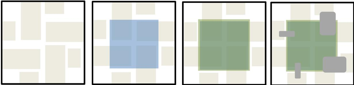
Figure 2 - Blank ITO, PEDOT layer, Polymer Layer, and Metal Cathode from left to right.
