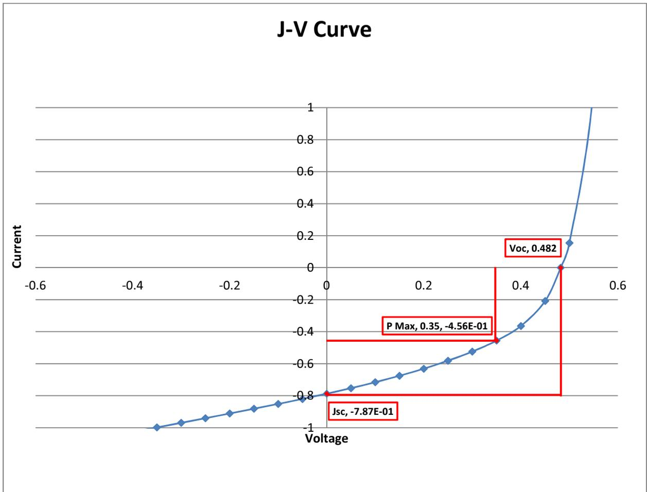
Figure 4 - J-V curve of a PCPDTBT device. The plot is scaled down to better represent the intersection of both axes. From a J-V curve we can calculate Jsc, Voc, Efficiency, and Fill Factor, see example calculations below:
