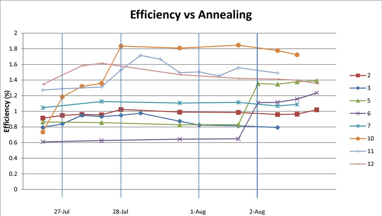
Figure 5 – Represents the effect of annealing on PCPDTBT and P3HT:PCPDTBT devices. The lines on certain dates represent the first anneal of the day while the markers represent the tests for a specific device. Some markers represent pre-anneal tests. Devices 5 and 6 were annealed last in accordance with Table 6 and showed significant improvement.
