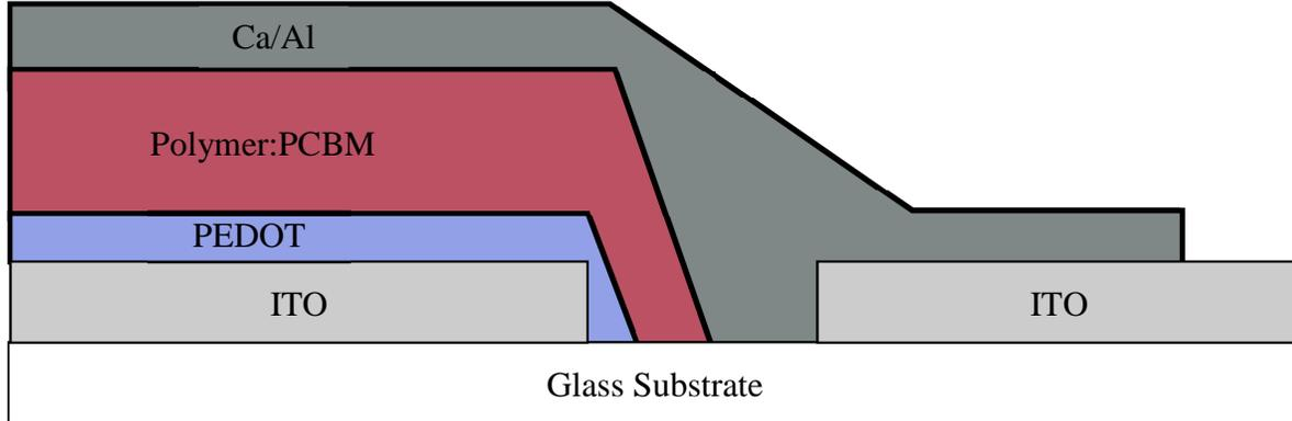
Figure 1 - A cross section of our devices, they are fabricated from bottom to top (Glass Substrate to Ca/Al cathode). This picture also shows the importance of wiping the Polymer:PCBM layer and PEDOT layer. Without wiping there would be a shorting pathway between the active layer ITO pad and the cathode. Additionally, without wiping the Polymer:PCBM layer adequate contact could not be made with the ITO.
