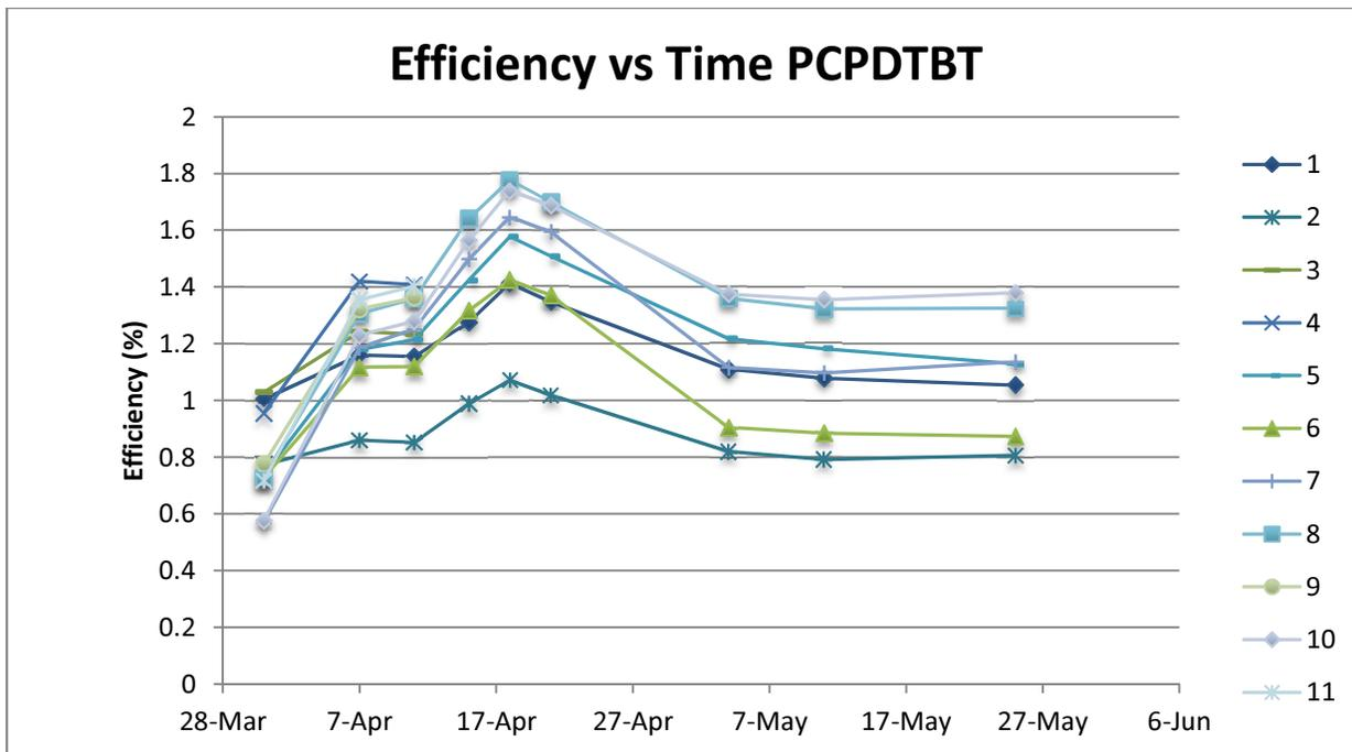
Figure 3a - The first PCPDTBT run showing efficiency through time. The initial rise is due to an increase in Voc, the second rise is due to a rise in Jsc which is currently unexplained. The devices begin to degrade as Jsc falls without any additional increase in Voc.
