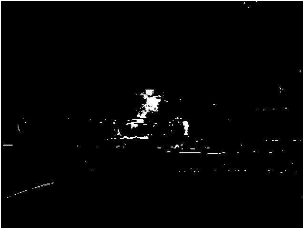
Figure 14: Binary difference image showing plume
