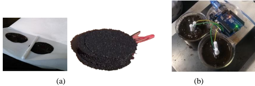
Figure 1. microbial fuel cell electrodes fabrication (b) electricity generation using electrodes and soil
