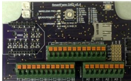
Figure 2. Wireless soil moisture sensor data acquisition board
