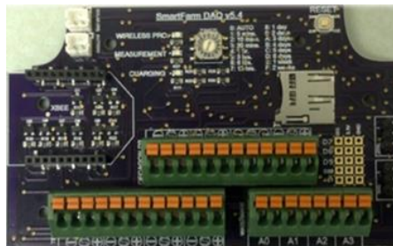
Figure 2. Wireless soil moisture sensor data acquisition board
