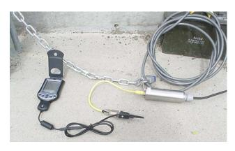
Figure 5. Telog PR-31 connected to the M125 Palm Pilot.
