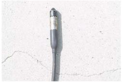
Figure 3. 5 psi Druck pressure sensor.
