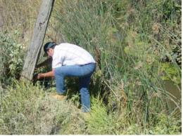
Figure 1. Installing a Telog PR-31 data collector at a spill site.
