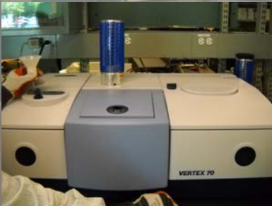
Infrared spectrometer, modified for emissions
