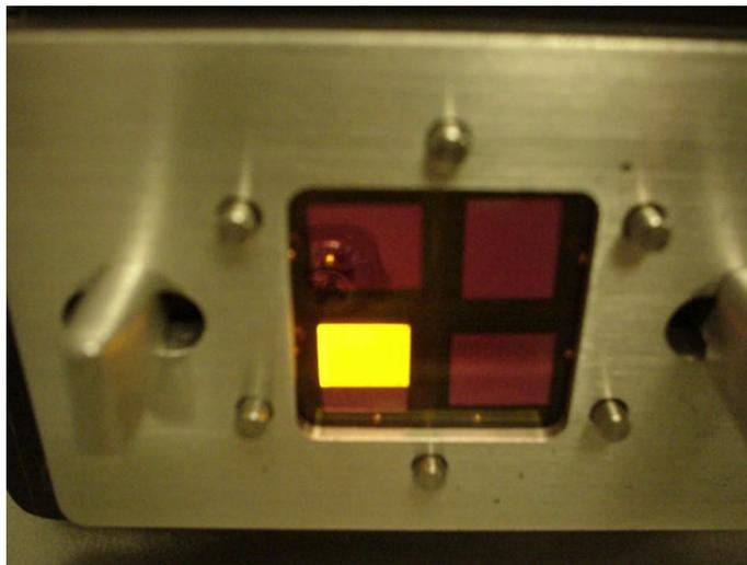
Figure 3 – Polymer LEDs in Test Jig<sup>2</sup>
