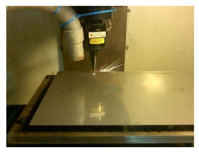
Figure 10 - CNC Laser Head Cutting Stainless Steel
