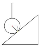
Figure 7 - Illustration of Ball Probe Error
