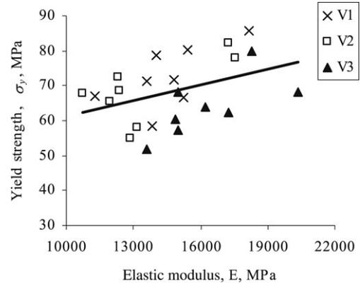
**Fig. 8 – Linear regression results of yield strength vs. elastic modulus for the 24 specimens. Regression parameters are slope: 0.002, intercept: 45.9 MPa, *p* < 0.050, *R*<sup>2</sup> = 0.16.**
