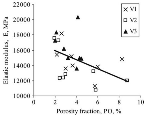
**Fig. 6 – Linear regression results of elastic modulus vs. porosity for the 24 specimens. Regression parameters are slope: –601.7, intercept: 17, 164 MPa, *p* = 0.022, *R*<sup>2</sup> = 0.22.**
