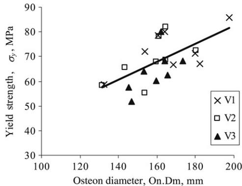
**Fig. 7 – Linear regression results of yield strength vs. osteon diameter for the 24 specimens. Regression parameters are slope: 0.361, intercept: 10.2 MPa, *p* = 0.002, *R*<sup>2</sup> = 0.37.**
