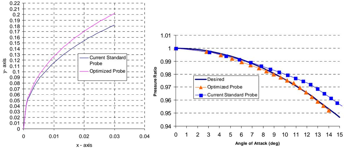
**Figure 12. Optimized probe shape and pressure distribution.**
