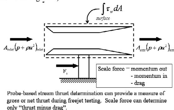
Figure 1. Static thrust measurements (Refs. 1 and 2).
