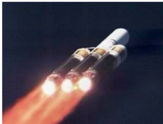
Fig. 1. Delta IV nozzle plume, at sea level (left), and at altitude. In the launch image, the plume is visibly overexpanded, evidence of a nozzle designed for optimum C_F at much higher altitudes [1].
