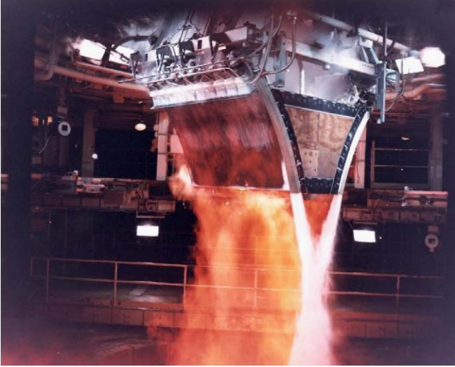
Fig. 3. X-33 truncated linear aerospike, during hot-fire test [4].
