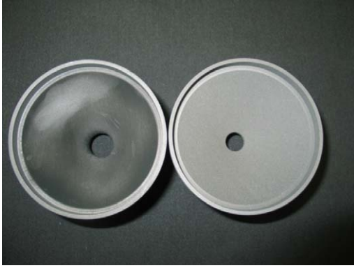
Fig. 4. Converging sections of conventional nozzle graphite liners, used in uncooled, hot-fired tests. The nozzle on the right is new; the one on the left has been fired for approximately 20 s. The severe ablation is evident, as shown by the increased area of the left throat. The thrust performance of the nozzle degraded continuously throughout the test; the nozzle is un-reusable.
