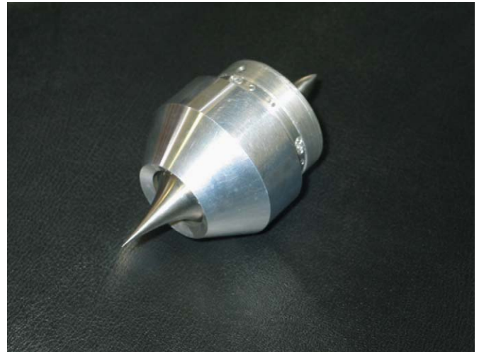
Fig. 2. Cal Poly's aerospike nozzle, used for cold flow tests.
