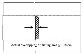
Figure 3. Carrier Rule for Manufacturer's Edge Overlap.
