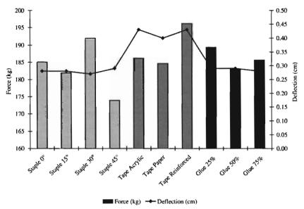
Figure 7. Compression Strength of Boxes with Different Types of Manufacturer Joints.
