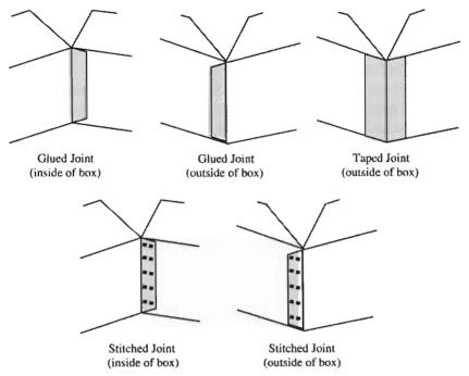
Figure 2. Common Styles of Manufacturer's Joints.
