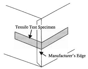
Figure 4. Tensile Test Specimen Location.
