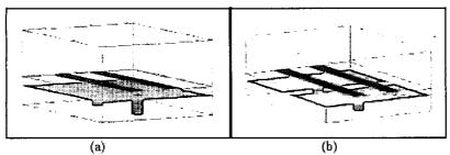
Figure 5 (a) 3-D view of a bidirectional microstrip transmission pair on a 10-mil thick bismalenmide trazine (BT) substrate, with a solid ground plane underneath. The ground plane is suspended above absolute ground and connected by vias to enable cleaving of the ground plane. (b) 3-D view of a bidirectional microstrip transmission pair on a 10-mil thick BT substrate, with a 10-mil cleave in the ground plane underneath.
