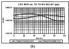
Figure 4 (a) The setup diagram for testing crosstalk penalty of a 10GB/s multiplexing/demultiplexing fiber optic transponder. (b) Bit error ratio variation of a 10GB/s multiplexing / demultiplexing fiber optic transponder as the transmitter to receiver delay is varied by one unit interval (100ps), measured at 25C and 70C.
