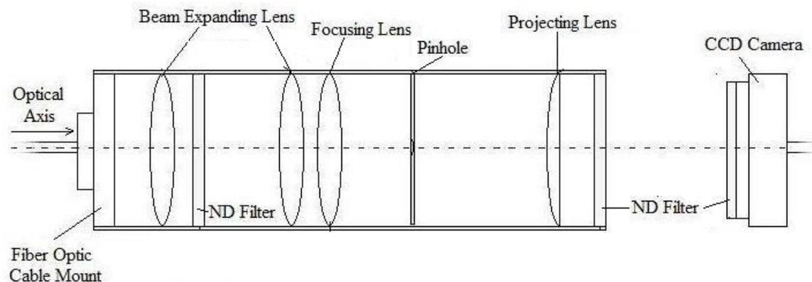
Figure 1. Theoretical set up for projected pinhole diffraction.
