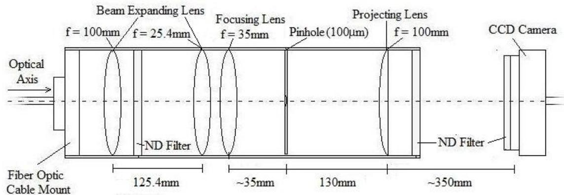
Figure 8. Experimental set up for projected pinhole diffraction
