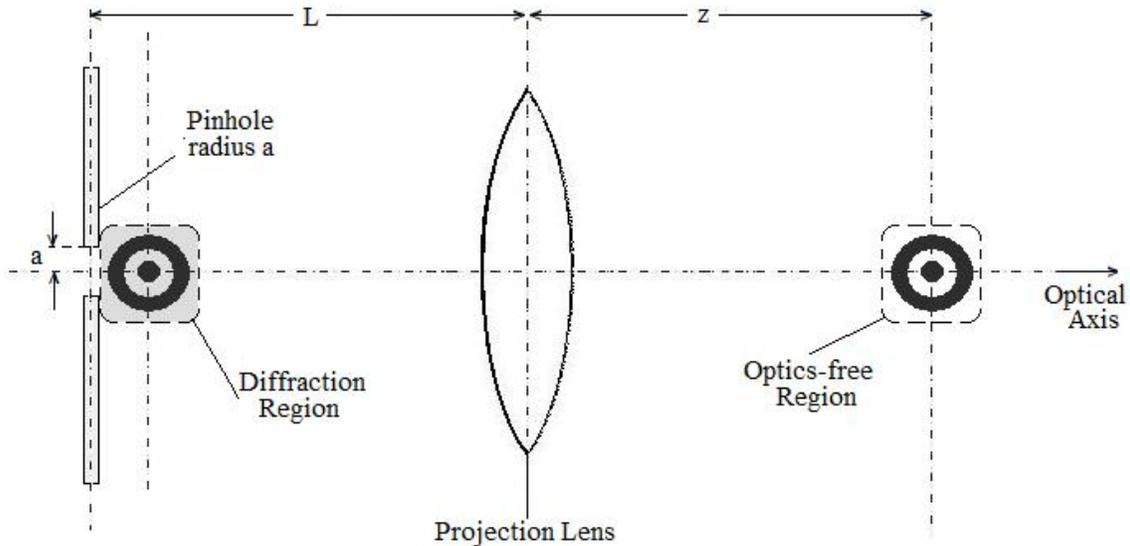
**Figure 7. Theoretical setup for projecting near-field diffraction patterns to an optics-free region**
