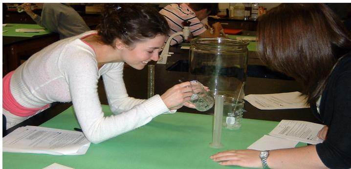
Student is amazed, or amused, by how fast a superabsorbent polymer absorbs water when the polymer particles are small.
