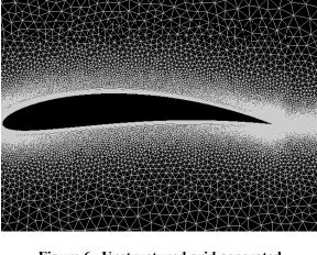
Figure 6. Unstructured grid generated about an NACA airfoil.
