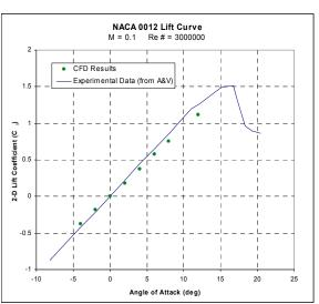
Figure 7. Comparison of CFD predictions with experimental data<sup>10</sup> for a NACA 0012 airfoil.
