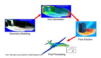
Figure 2. The Four Step CFD Process.
