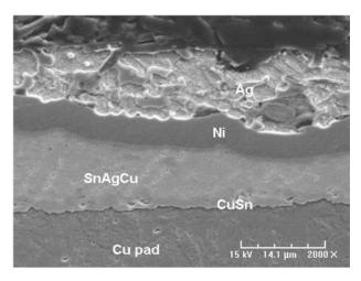
The component size in both figures is 0603. They show that the Sn layer in the chip component metallization was dissolved in the bulk SnPb or SnAgCu joints; a CuSn intermetallic compound (IMC) layer was formed between the bulk solder and the Cu pad and a thin NiSn IMC layer was formed between the bulk solder and the component. They also show the Ag layer
