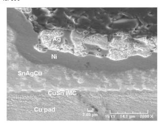
above the Ni layer. The fractures occured partially in the Ag layer and partially in the bulk solder joint, which implies that the shear strength of solder joint is higher than or equal to that of the component metallization.
