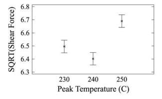
peak temperature of 250°C results in the highest shear force, while there is no significant difference in shear force between the peak temperature of 230°C and 240°C. Figure 7 shows that a TAL of 30 s results in the highest shear force, while there is no significant difference in shear force between the TAL of 60 and 90 s.
