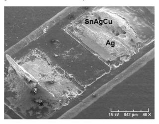
Figure 14 Typical termination structure of a lead free chip resistor
