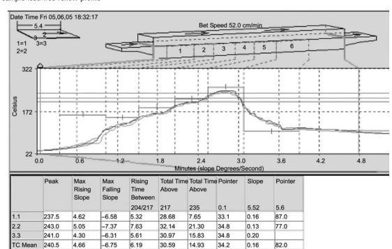
Figure 2 A sample lead-free reflow profile
