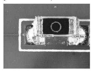
Figure 11 Fracture area of a SnPb joint reflowed at 195°C for 30 s
