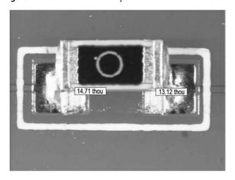
Figure 12 Fracture area of SnPb joint reflowed at 215°C for 90 s
