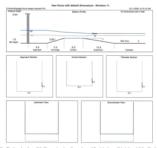
Figure 6. Profile drawing from WinFlume showing dimensions of final design. sill height = 1.8 ft, sill width = 8.2 ft.
