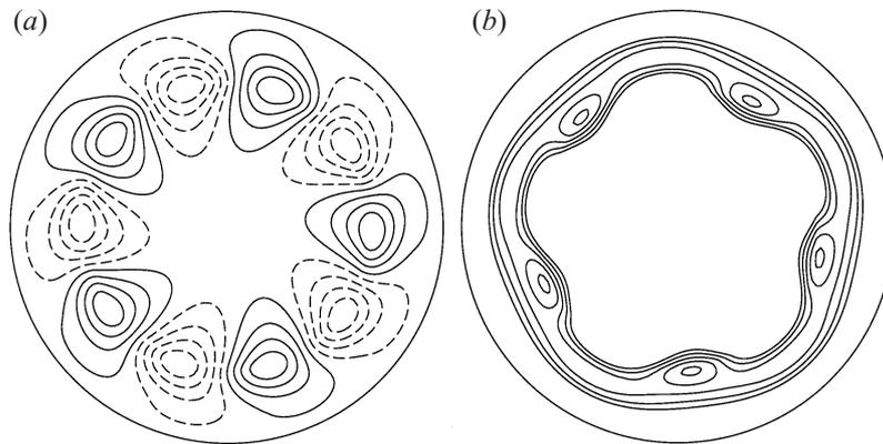
FIGURE 3. The spatial form of the most unstable mode shown in figure 2 ( $n = 5$ ). Parameters are  $\mu = 1$ ,  $r_{max} = 2\pi$ ,  $a = 0.75$  and  $r_0 = 2\pi - 2a$ . (a) Upper-layer stream function or geostrophic pressure (the contour interval is 0.066); (b) lower-layer height (the contour interval is 0.3). Dotted lines indicate negative values.
