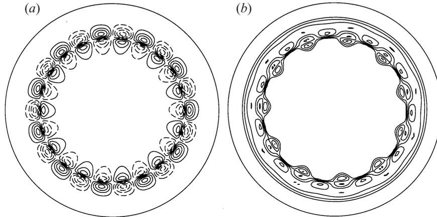
FIGURE 5. The spatial form of the most unstable dipole mode at  $\mu = 10$  ( $n = 11$ ). Parameters are  $r_{max} = 2\pi$ ,  $a = 0.75$  and  $r_0 = 2\pi - 2a$ . (a) Upper-layer stream function or geostrophic pressure (the contour interval is 0.0066); (b) lower-layer height (the contour interval is 0.26). Dotted lines indicate negative values.
