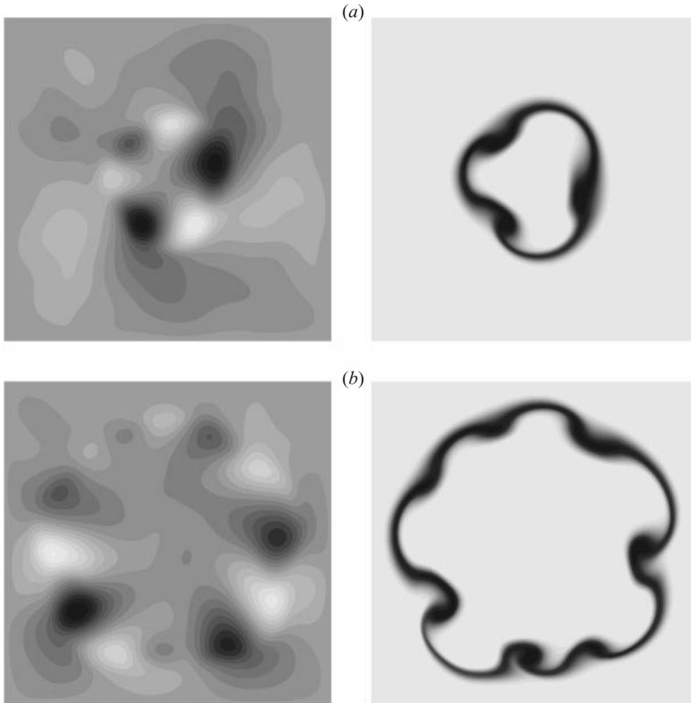
FIGURE 13. Upper-layer stream function (left) and lower-layer height (right) for runs identical to the one shown in figure 11, except that  $r_{max} = 7.5$  and  $r_0 = 3$  (a) and  $r_0 = 6$  (b).  $r_0 = 3$  run shown at  $t = 12$ , and  $r_0 = 6$  run shown at  $t = 10$ . Darker shades denote larger values. Lower-layer ranges are  $(0.0, 0.94)$  and  $(0.0, 0.97)$ , and upper-layer ranges are  $(-0.34, 0.48)$  and  $(-0.57, 0.79)$ , for  $r_0 = 3$  and  $r_0 = 6$ , respectively.
