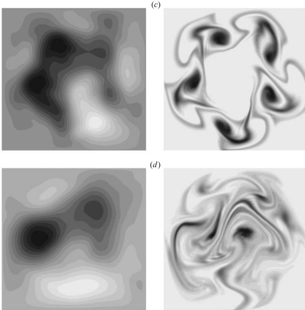
FIGURE 11(c, d). Upper-layer stream function (left) and lower-layer height (right) at times  $t = (a)$  0,  $(b)$  10,  $(c)$  20 and  $(d)$  40. Darker shades denote larger values. Lower-layer ranges are (0.0, 1.0), (0.0, 0.96), (0.0, 0.96), (0.0, 0.84), and upper-layer ranges are  $(-0.07, 0.07)$ ,  $(-0.52, 0.65)$ ,  $(-0.74, 0.9)$  and  $(-1.05, 1.89)$  for times 0, 10, 20 and 40, respectively.
