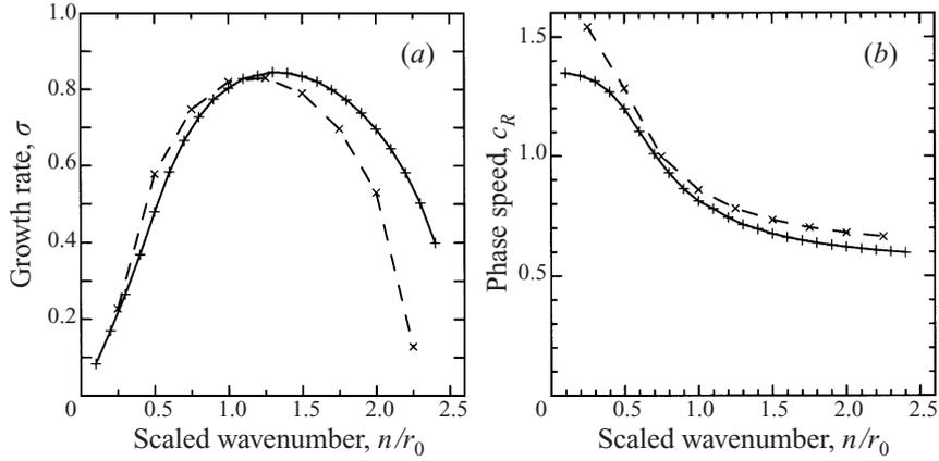
FIGURE 8. Growth rate and phase velocity versus scaled wavenumber  $n/r_0$  for  $r_0 = 4$  (dashed lines,  $\times$ ) and  $r_0 = 10$  (solid lines,  $+$ ). Parameters are  $\mu = 2$ ,  $a = 1$  and  $r_{max} = r_0 + 2a$ .
