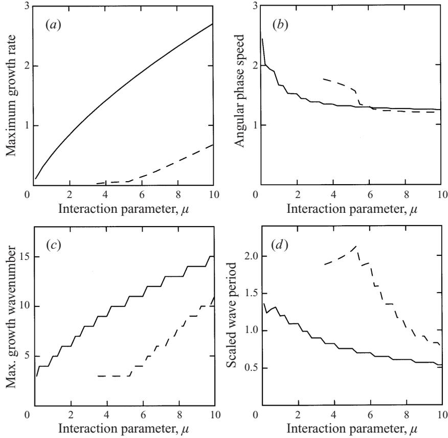
FIGURE 4. Dependence of disturbance characteristics upon interaction parameter  $\mu$ . Other parameter values are  $r_{max} = 2\pi$ ,  $a = 0.75$  and  $r_0 = 2\pi - 2a$ . Solid line represents the monopole mode, dashed line represents the dipole mode. Wavenumber discretization is the cause of the jagged appearance of some of the plotted lines.
