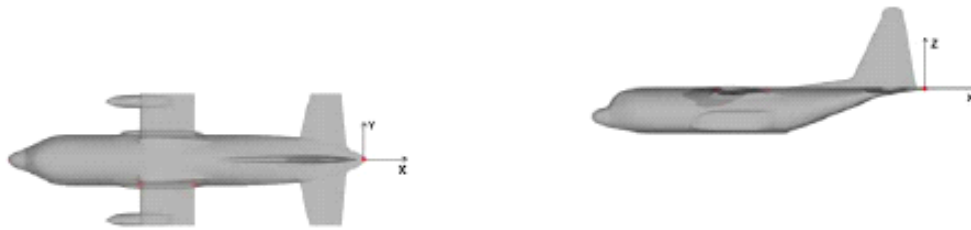
Figure 3: C-130 Model Datum point (courtesy of ENSICA)
