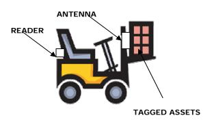
FIGURE 5. RFID SET-UP FOR FORK LIFT TRUCK.
