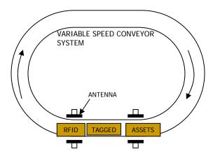
FIGURE 3. CONCEPTUAL DESIGN OF RFID CONVEYOR TRACKING SYSTEM.
