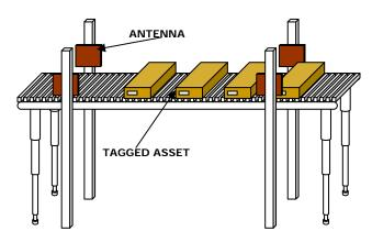
FIGURE 2. RFID SET-UP FOR CONVEYOR TRACKING SYSTEM.
