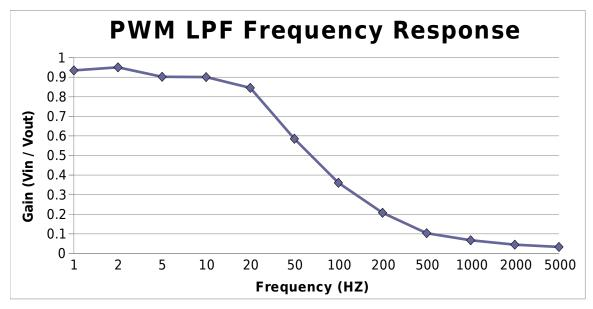
Figure 5: Measured PWM transfer characteristic
