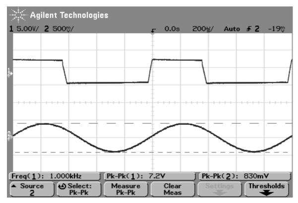
Figure 22: Fuzz circuit final output
