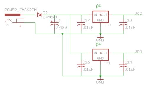
Figure 23: Power Supply Schematic
