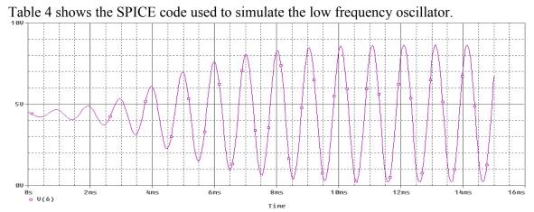
Figure 13: Low Frequency Oscillator PSPICE Simulation. V(6) is the output of the LFO.
