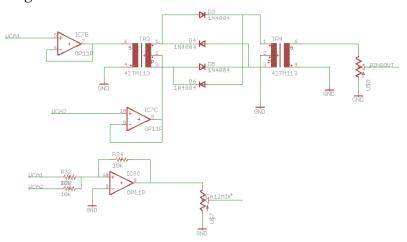
Figure 18: Ring Modulator Schematic
