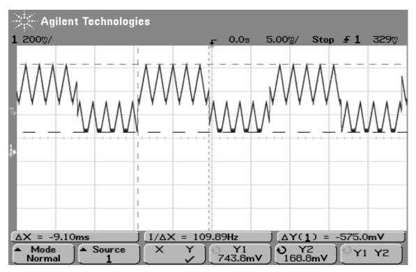
Figure 19: Mixed inputs from VCA1 and VCA2
