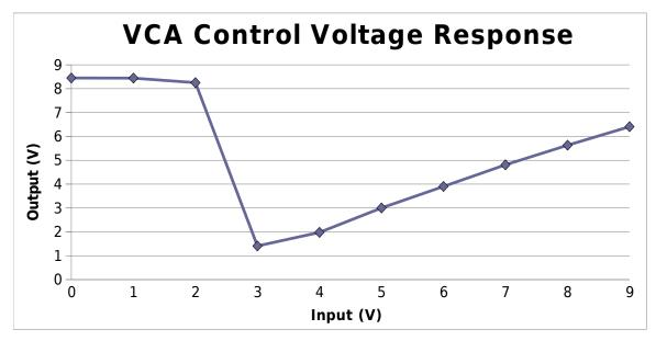
Figure 17: Voltage Controlled Amplifier Measured response
