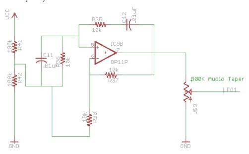
Figure 12: Low Frequency Oscillator Schematic
