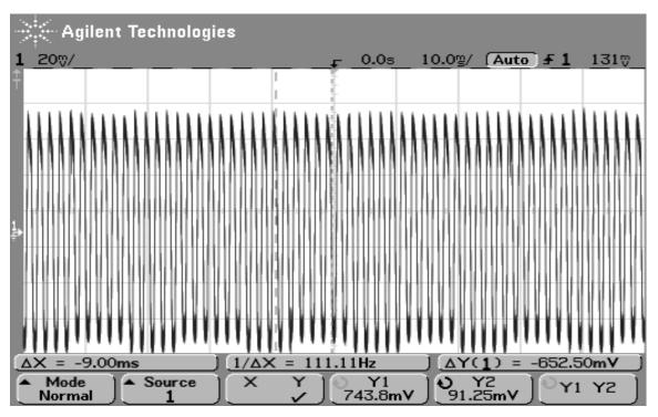
Figure 20: Ring Modulated inputs from VCA1 and VCA2
