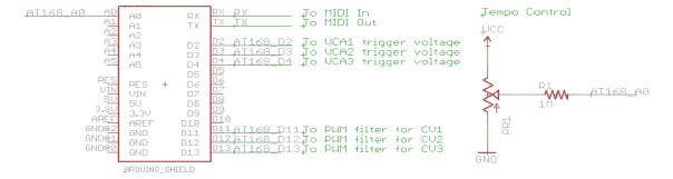
Figure 2: Atmega168 inputs and outputs
