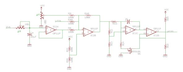
Figure 7: Voltage Controlled Oscillator Schematic
