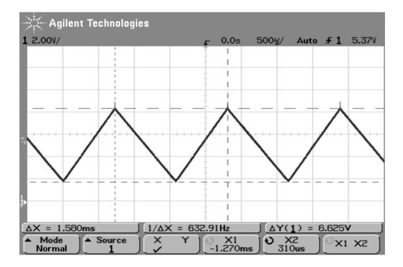
Figure 10: VCO Triangle Wave Output
