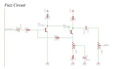
Figure 21: Fuzz Circuitry and Output Volume Schematic
