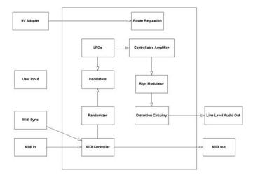
Figure 1: Project Block Diagram
