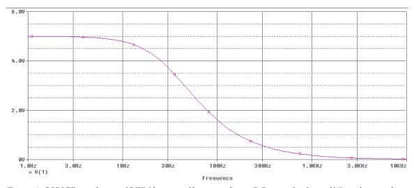
Figure 4: PSPICE simulation of PWM low pass filter providing a DC control voltage. V(1) is the transfer characteristic of the low pass filter with a 5V input at varying frequencies.
