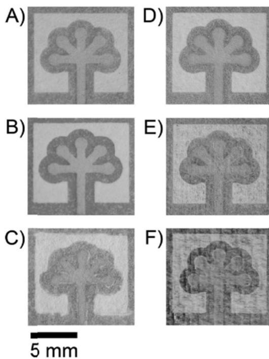
**Fig. 3** Micro-PADs produced using chromatography paper by (A) printing the pattern with an ink-jet printer, (B) printing the pattern with a photocopy machine, and (C) drawing the pattern through a stencil using a waterproof black pen. A  $\mu$ PAD patterned using sunlight (D). A  $\mu$ PAD from Technicloth (E), or a paper towel (F). The devices were filled with an aqueous blue dye (1 mM Erioglaucine).
