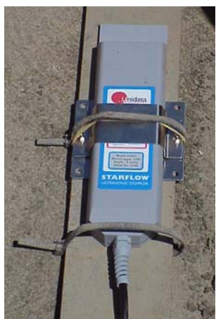
Figure 2. Unidata STARFLOW Ultrasonic Doppler Flow Meter, secured to 1/4" steel plate to anchor it on the canal floor.
