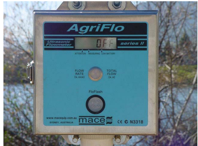
Figure 7. The electronics module of the MACE Agriflo
