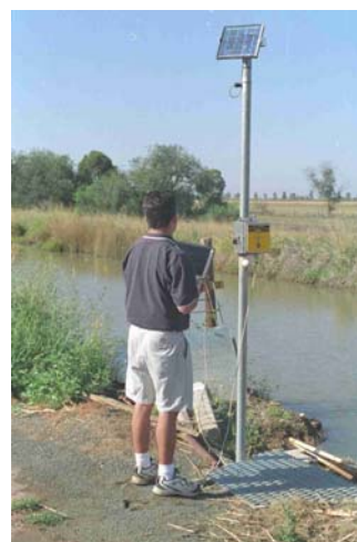
Figure 8. Collecting data from a MACE Agriflo Doppler Flow meter
