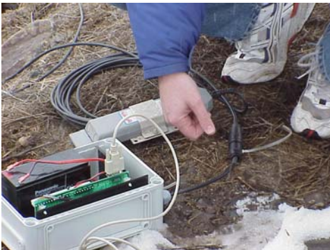
Figure 3. STARFLOW sensor connected to MicroLogger box, Kittitas ID. Note the battery and the communications cable connecting the MicroLogger to a laptop computer.
