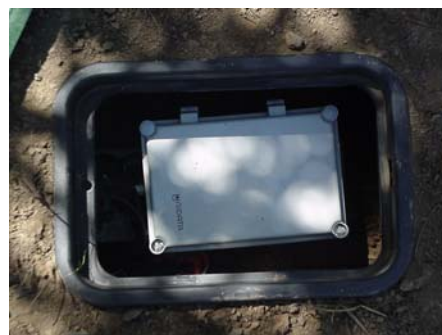
Figure 4. MicroLogger in buried irrigation valve box, Sutter-Mutual WC. The unit sits on a masonry brick to keep it off the ground.
