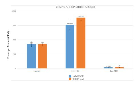
Figure 4: CPM ( $\pm$  S.E.) comparison between Al-HDPE and HDPE-Al shield orientations for Co-60, Cs-137 and Po-210. Only Cs-137 produced a difference (p < 0.05) in shield effectiveness based on orientation.
