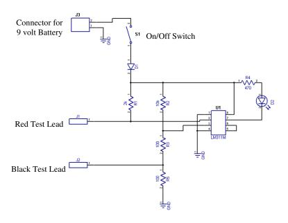
Figure 1 Schematic of Continuity Tester
