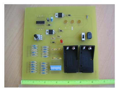
Figure 3 Prototype op-amp PCB for Laboratory Learning Module
