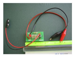
Figure 2 Top View of Continuity Tester
