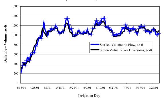
Figure 5. Daily Flow Volume in the Tisdale Main Canal (Tisdale Bridge) measured by the SonTek Argonaut<sup>TM</sup> SL compared to the calibrated flows of the Tisdale Pumping Plant.
