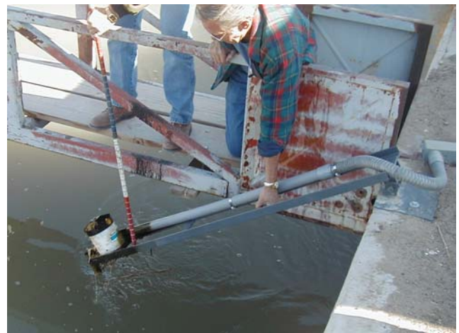
Figure 5. Mounting hardware for Argonaut SL at Truckee-Carson Irrigation District
