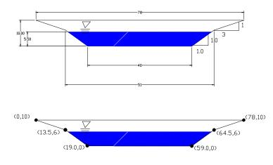
Figure 4. Tisdale Main Canal Cross Section
