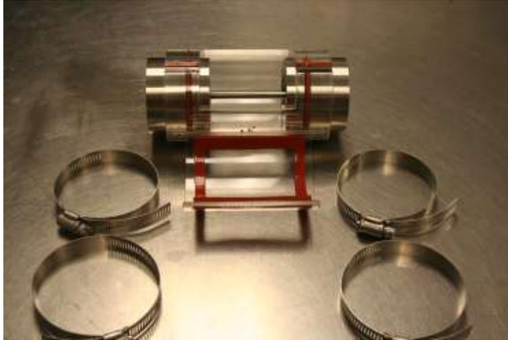
**Figure 8: Bioreactor prototype.** In the image can be seen the hose clamps with the screws that tighten the housing around the stainless steel parts. The viewport window can be seen cut into the acrylic housing including the silicon gasket around the edge.
