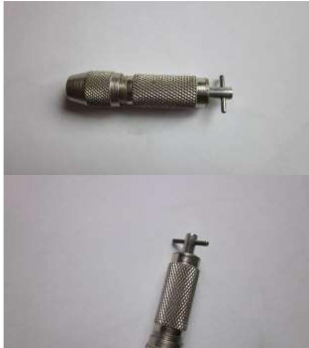
Figure 14: The top image shows the pin vise that was modified to fit into the electrospinning machine interface. The bottom image shows the pin that was put through the diameter of the pin vise to allow for the spinning drive to spin the mandrel.
