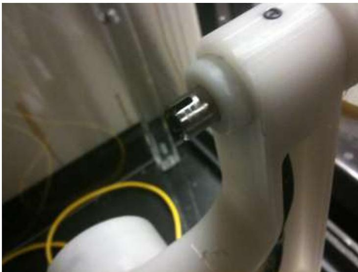
Figure 13: The interface end that drives the pin end of the mandrel and spins the mandrel.
