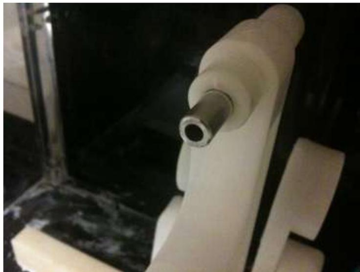
**Figure 12:** Live centering interface of the electrospinning machine. The pin that acts to center the mandrel is within the cylinder shown in the image.
