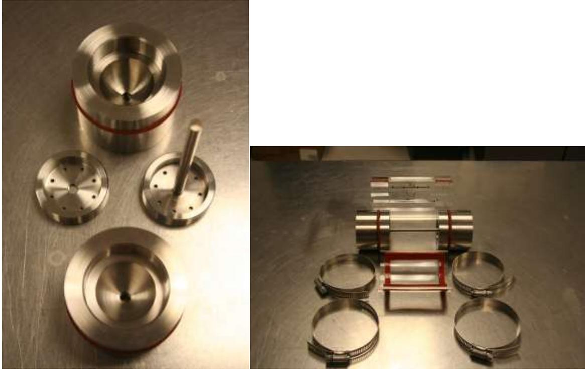
Figure 9: To the left is an image of the stainless steel parts. At the top and bottom are the endcaps. In the middle are the scaffolding caps which will hold the scaffolding. The image on the right is all of the parts to the bioreactor disassembled.
