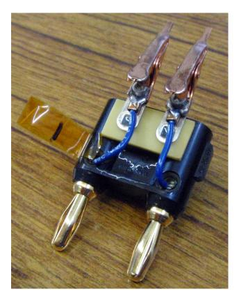
Figure 5. Photo of a Fuse Holder.
