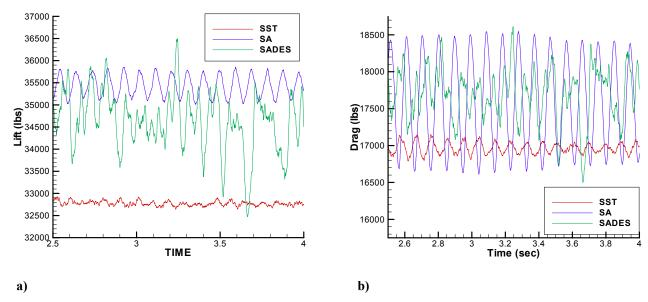
Figure 11. Time histories of the a) Lift force and b) Drag force in lbs for the SST, SA, and SADES methods
