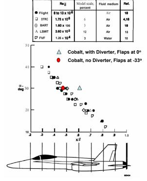
Figure 10. Streamwise LEX vortex breakdown position as a function of angle of attack, extracted from Ref. 47 SADES mean vortex breakdown position in red.
