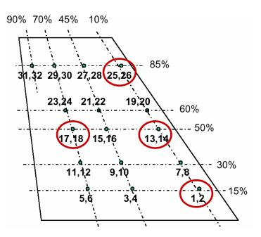
Figure 13. Placement of the F-18 HARV Kulite pressure sensors on the right vertical tail.<sup>47</sup> Odd port numbers are on the inboard section of the tail and even are on the outboard section. Red circles around ports indicates those used in comparing flight test to SADES.
