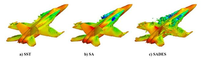
Figure 8. Isometric views of the F/A-18C at  $\alpha = 30^{\circ}$ , Re<sub>c</sub> = 13 x10<sup>6</sup>, leading edge flaps set to -33°, trailing edge flaps set to 0°, with no diverter slot present: a) SST turbulence model, b) SA turbulence model, and c) SADES turbulence model.
