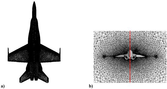
Figure 7. a) Top View of the Baseline Grid (3.9 million cells). b) Baseline grid of 3.6 million cells (left) and AMR grid of 3.9 million cells (right) at a station 450 inches aft of the origin. Darkened regions above the LEX show adapted mesh refinement of the vortex.
