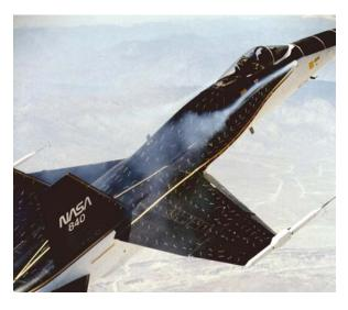
Figure 1. NASA F-18 High Angle of Attack Research Vehicle (HARV). Photo Courtesy of NASA Dryden.
