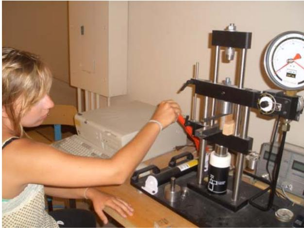
**Figure 1. Shear Testing of Composite**
