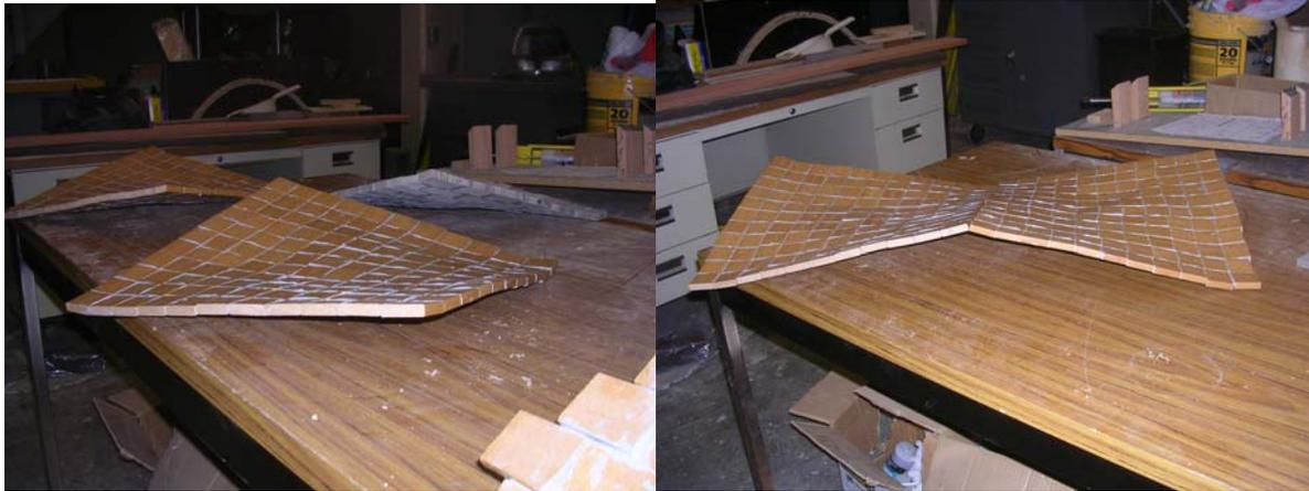
**Figure 3. Modular Hyperbolic Paraboloids Made of Composite**
