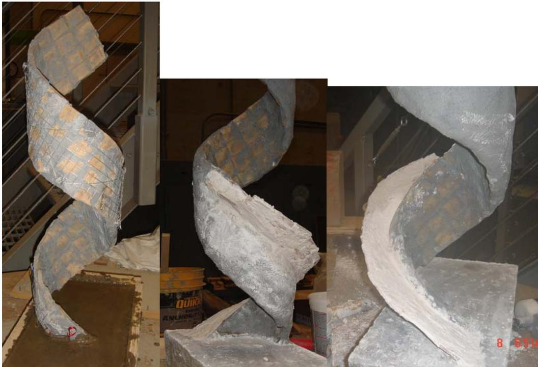
**Figure 4. Benchtop Scale Spiral Staircase Made of Composite**
