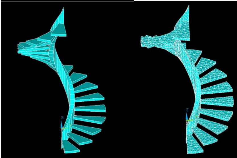
**Figure 5. Finite Element Models of Spiral Staircase**
