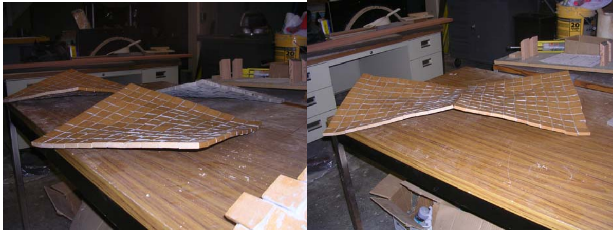
Figure 3. Modular Hyperbolic Paraboloids Made of Composite
