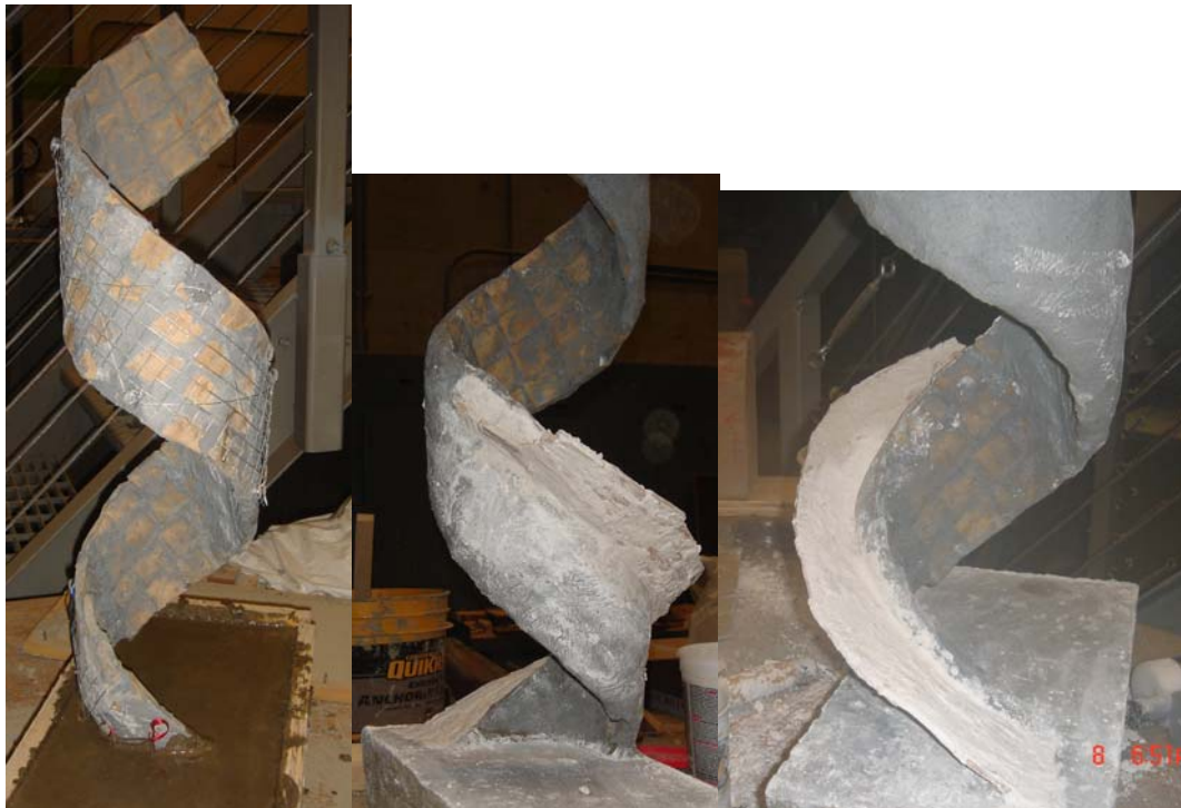
Figure 4. Benchtop Scale Spiral Staircase Made of Composite
