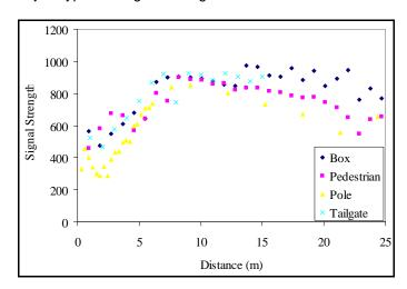
Figure 10: LIDAR signal strength as a function of distance for various objects in static tests
