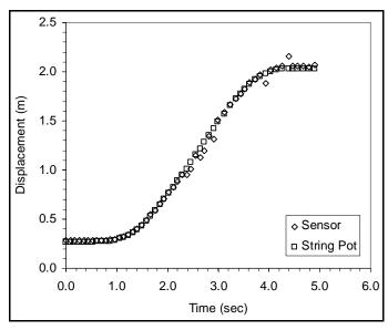
Figure 8: Typical results for dynamic test of ultrasonic sensor compared with string pot.
