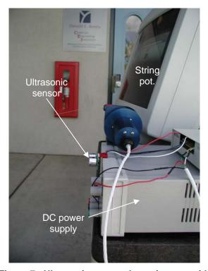
Figure 7: Ultrasonic sensor dynamic tests with string pot.
