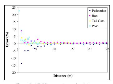
Figure 5: LIDAR percent error in distance measurement as a function of distance for various objects in static tests
