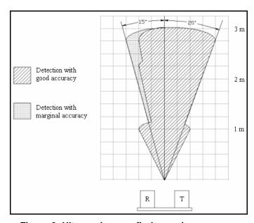
Figure 2: Ultrasonic rangefinder sonic cone map
