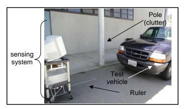
Figure 6: Experimental setup for multiple object static testing used in all sensor types
