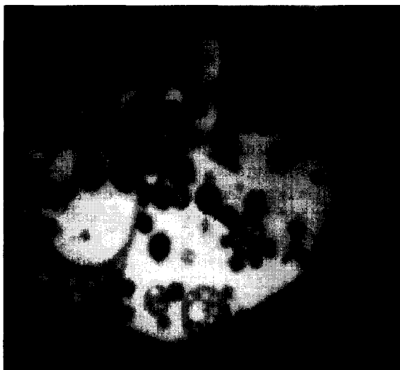
Fig. 1. Fluorescence micrograph of monolayer showing coexisting DChol-rich (gray), phospholipid-rich (white), and gas (black) phases.
