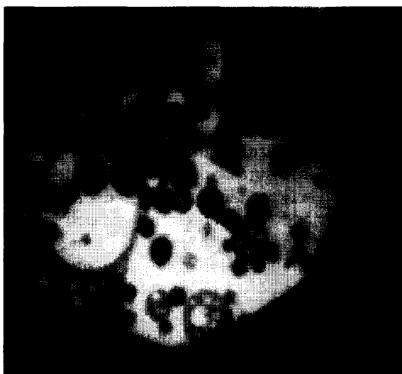
Fig. 1. Fluorescence micrograph of monolayer showing coexisting DChol-rich (gray), phospholipid-rich (white), and gas (black) phases.
