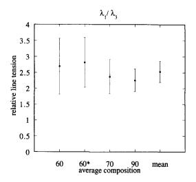
Fig. 5. Relative line tension,  $\lambda_1/\lambda_3$ , at different system compositions. Line tension is unaffected by system composition. The composition numbers refer to the mol% DChol. 60\* refers to data taken from gas domains of case I morphology. All other data were taken from gas domains of case II morphology. Data are shown with 95% confidence intervals.
