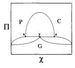
Fig. 4. Schematic of the lipid/DChol phase diagram. P is the phospholipid-rich phase, C is the DChol-rich phase, G is the gas phase,  $\Pi$  is the surface pressure, and  $\chi$  is the composition (mole fraction DChol). x, y, and z are the compositions of the three coexisting phases.
