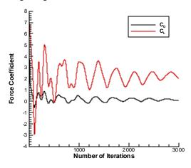
Figure 7. Convergence history for grid created with adaptive mesh refinement.
