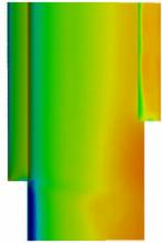
Figure 11. Surface pressures for part-span flap configuration.
