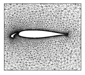
Figure 4. Spanwise cut of unstructured grid for wing at y/b = 0.25.
