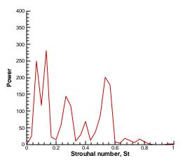
Figure 14. Power spectrum density of wing lift.
