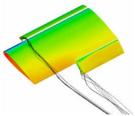
Figure 12. Surface pressures and slat/flap vortices for part-span flap configuration.
