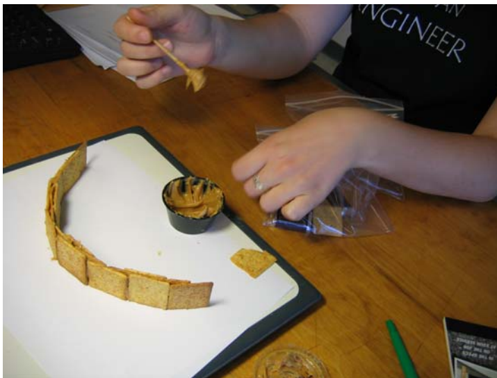
Figure 8. Laminated arch being constructed on its side
