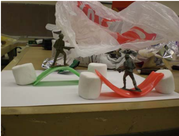
Figure 5a. One arch and one beam
