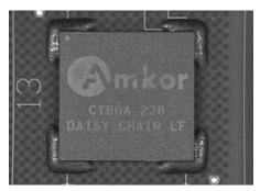
Figure 1. An example of an edge-bonded CSP.
