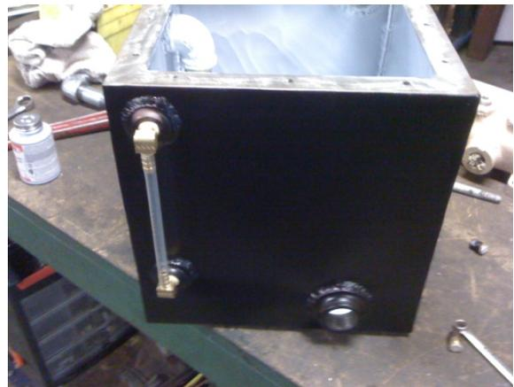
**Figure 9. Sight gauge and tank coating**
