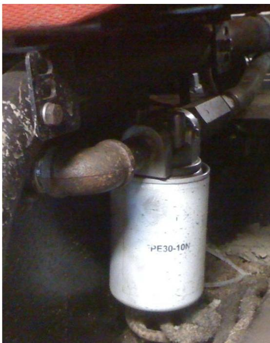
**Figure 10. Filter and Check Valve**
