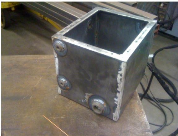
**Figure 8. Hydraulic Reservoir under construction**
