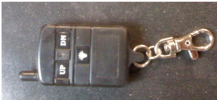
**Figure 11. Wireless winch control**
