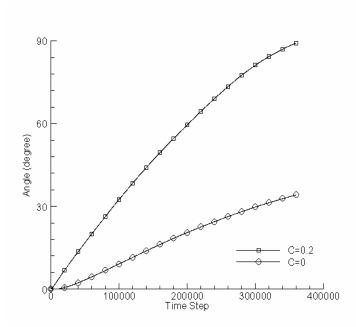
Figure 8: Rotation angles of curved and straight fiber at density ratio of 1.001 and Reynolds number around 1.3
