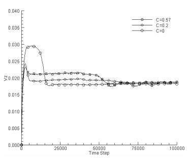
Figure 9: The terminal velocities of curved and straight fibers at the same density ratio of 1.05 are the same. However they have different trajectories. The Reynolds number of straight fiber is Re=37.7, the Reynolds number for curved fiber is Re=31.2. The concave surfaces of curved fibers are towards the left wall in this case
