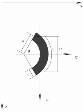
Figure 1: Curved fiber and its parameters
