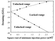
Fig. 2 Locking range dependence on both injected power and detuning for a fixed test laser bias of 30 mA at 25 °C.
