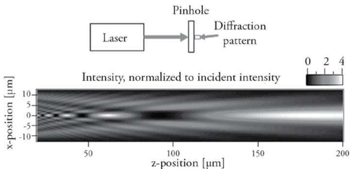
**Figure 3.** The diffraction pattern created by light incident on an aperture [5].
