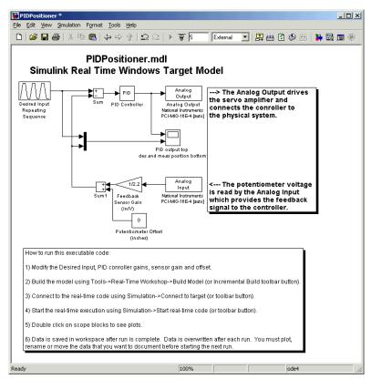
Figure 3. Closed-Loop PID Controller Interface
