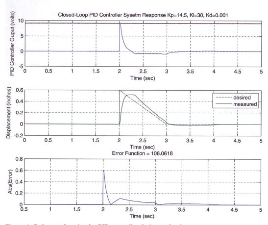
Figure 6. Reference function for PID controller design evaluation
