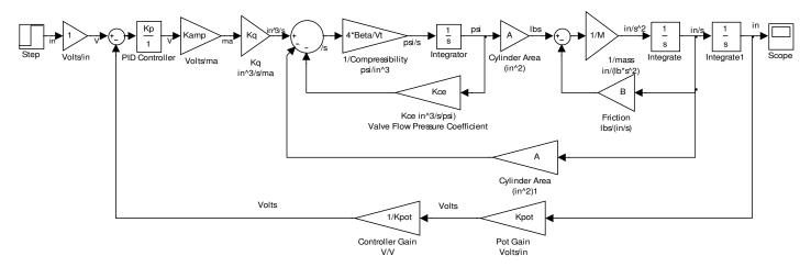
Figure 4. Simulink model of closed-loop hydraulic servo control system
