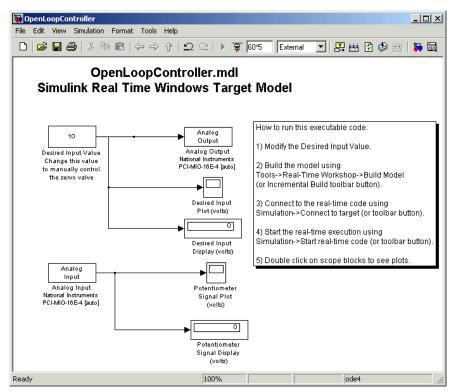
Figure 2. Open-Loop Controller RTWT Interface
