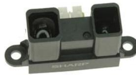
Figure 1: SHARP GP2Y0A700K distance module
