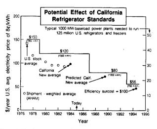
Fig. 2. California Mandatory Refrigerator Standards reduce the average energy intensity from 1900 kW h/yr in 1977 to  $700 \, kW$  h/yr in 1993. The operating costs have been calculated with an electricity price of 8 ¢/kW h. The number of 1-GW base-loaded power plants needed to run the nation's 125 million refrigerators and freezers is displayed on the right-hand scale. (A. Rosenfeld, Ref. 3, p. 103.)
