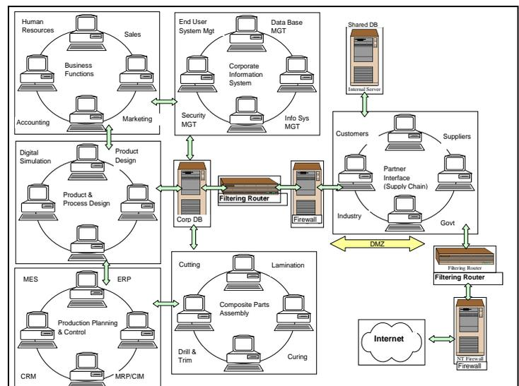
Figure 4. Configuration of a seamless integrated information system
