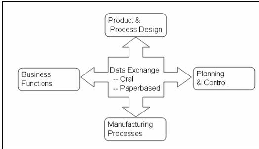
**Figure 1.** Data Communication in Traditional Paper-based Manufacturing Industry
