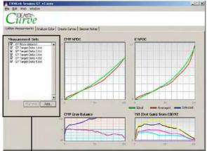
Figure 2: Un-calibrated curves of gray balance and TVI.
