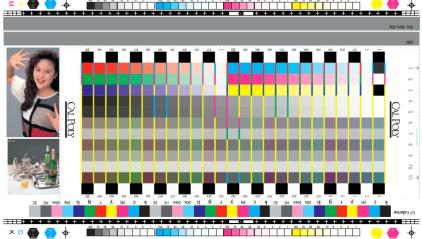
Figure 1: Designed test target for calibration.
