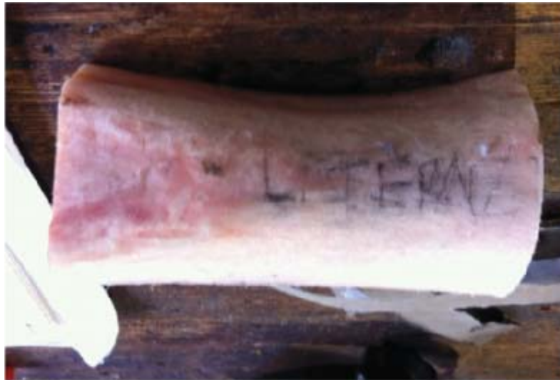
Figure 5a —Labeling of the lateral face of the bovine femur after all the excess tissue and meat has been scraped off, and the two epiphyses ends have been cut off.
