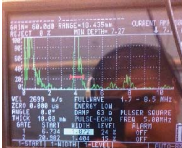
Figure 15 — The screen of the Panametrics NDT Ultrasound machine as it subjects a bone sample to ultrasonic testing. The peak on the left is noise from the transducer as it sends the signal through the bone. The second peak is the result of the sound waves coming back to the transducer. The red bar is “gate 1,” this gate will be used to measure the width of the top of the second peak.
