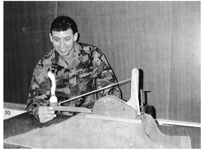
Fig. 5. The class applies the work-energy and projectile motion equations to determine the firing distance for the flaming catapult.
