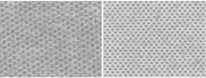
Figure 2: Laser engraved masterscreen black cells (left) and electromechanically engraved black cells (right).
